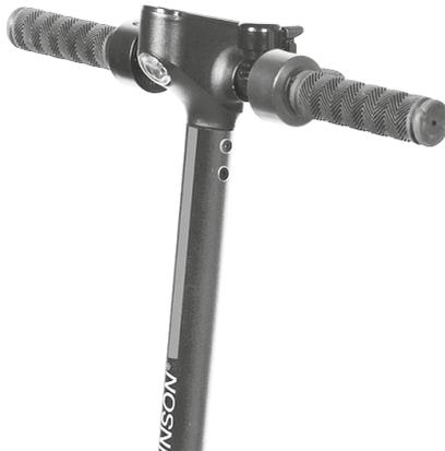
After matching the holes in the handlebar with those of the frame, insert the screws and tighten them well; repeat the operation also on the opposite side of the handlebar inserting a total of 4 screws.
